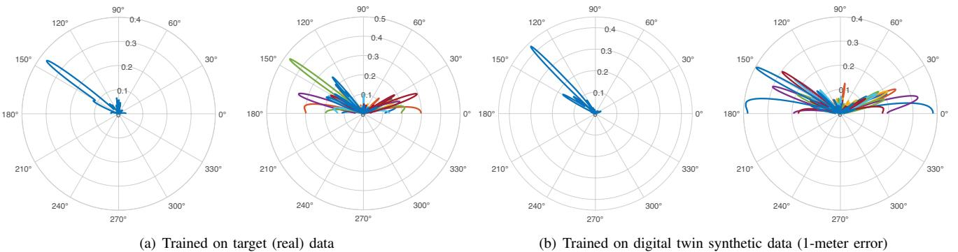
Fig. 4. This figure shows the beam patterns of the measurement vectors learned by the channel encoder. The number of measurement vectors is set to  $\{1, 8\}$ . Fig. 4(a) shows the learned beam patterns by the model trained on the target data, while Fig. 4(b) presents the learned beam patterns by the model trained on the digital twin data.
