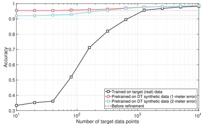
Fig. 5. This figure presents the prediction accuracy of the RF precoder with different numbers of real-world data points. The model is pretrained on 10240 synthetic data points and then fine-tuned on real-world data.
