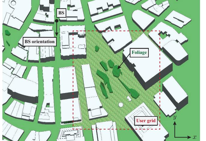
Fig. 2. The figure shows the adopted target scenario, which is built based on a section of downtown Boston. The base station is placed along a vertical street, while the foliage is represented by the dark green objects in the layout. The user grid is highlighted by the red box.
