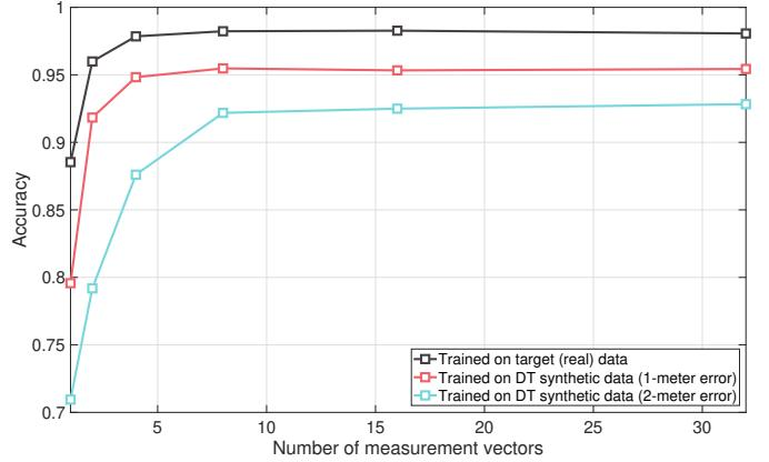
Fig. 3. This figure presents the prediction accuracy of the RF precoder with different numbers of measurement vectors. We consider the number of measurement vectors to be set to  $\{1, 2, 4, 8, 16, 32\}$ .
