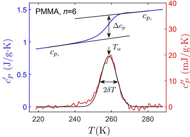
FIG. S1. TMDSC results for PMMA ( $n = 6$ ) across the glass transition, using a modulation period of  $P = 60$  s and an amplitude of  $A = \pm 1$  K.
