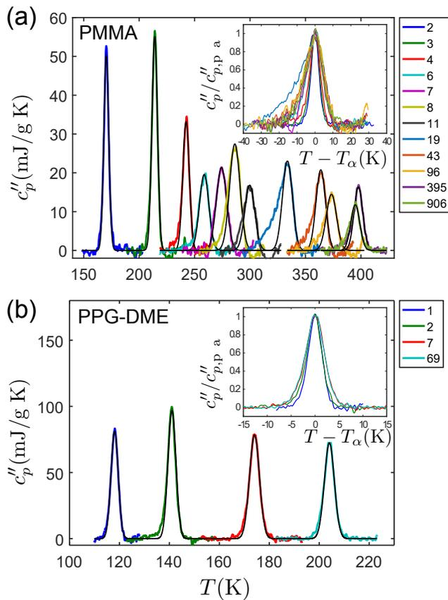
FIG. 1. The imaginary part of the  $T$ -dependent specific heat  $c_p''(T)$  for (a) PMMA and (b) PPG-DME. The legends show the degree of polymerisation  $n$ . The peak in  $c_p''(T)$  corresponds to the response due to the structural  $\alpha$  relaxation, with Gaussian fits (black lines). The insets show all  $c_p''(T)$  data normalized and centered on the peak temperature  $T_\alpha$ .
