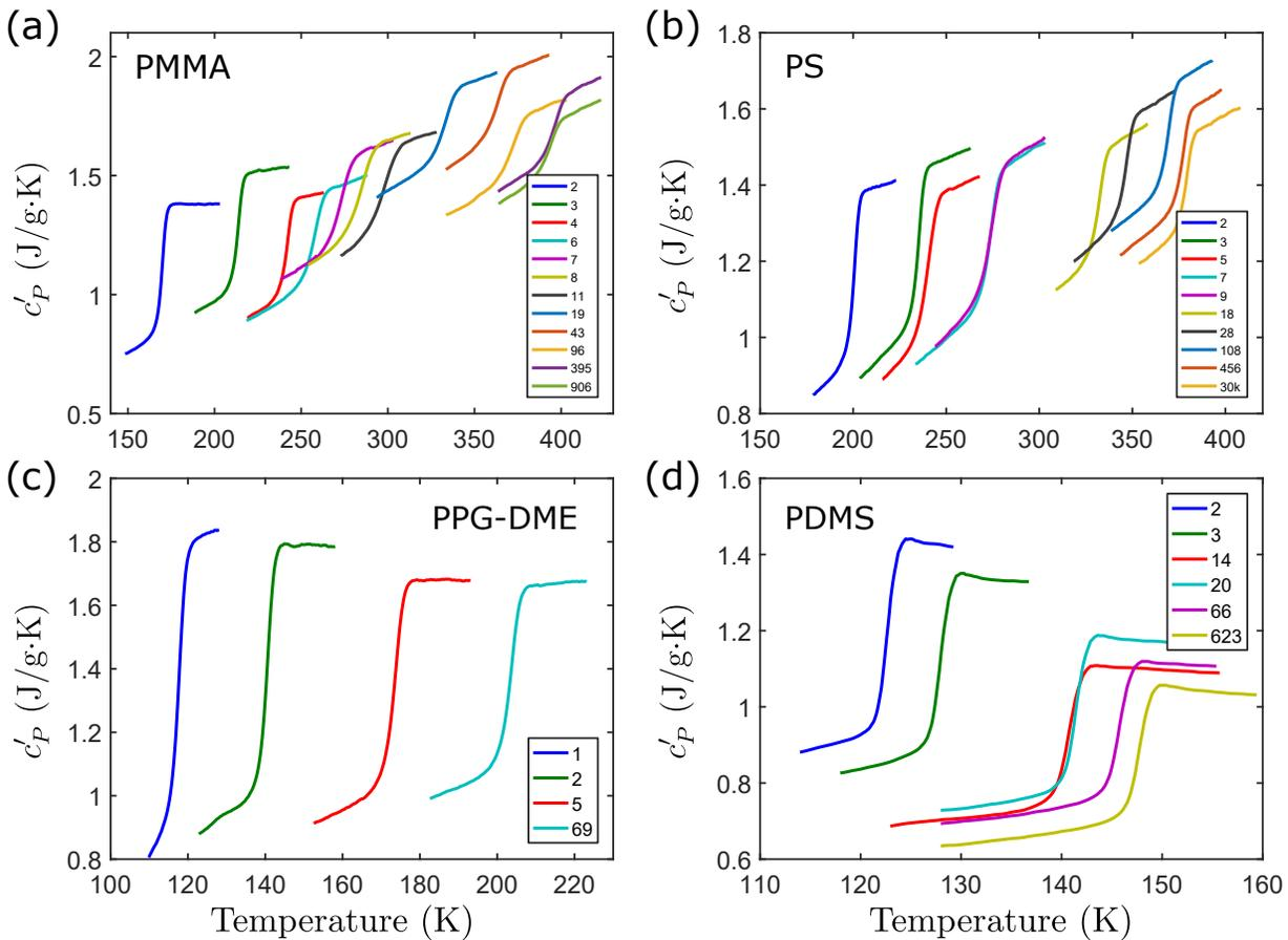
FIG. S2. The real part  $c'_P$  of the specific heat response at  $\omega = 2\pi/60 \text{ s}^{-1}$  for the four polymers. The degrees of polymerization  $n$  are shown in the legends.
