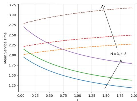
Figure 3. Mean service time  $\bar{T}_1$  vs  $\lambda$  for  $N = 3, 4, 5$  servers with service times  $\mu_i = 1.5$  for  $i = 1, \dots, N - 1$  and  $\mu_N = 1.5, 5,$  and  $10$  for  $N = 3, 4,$  and  $5$ , respectively. The solid and dashed lines indicate the mean service times under preemption and non-preemption, respectively.
