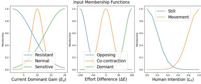
Fig. 2: Designed membership functions for the two controllers.
