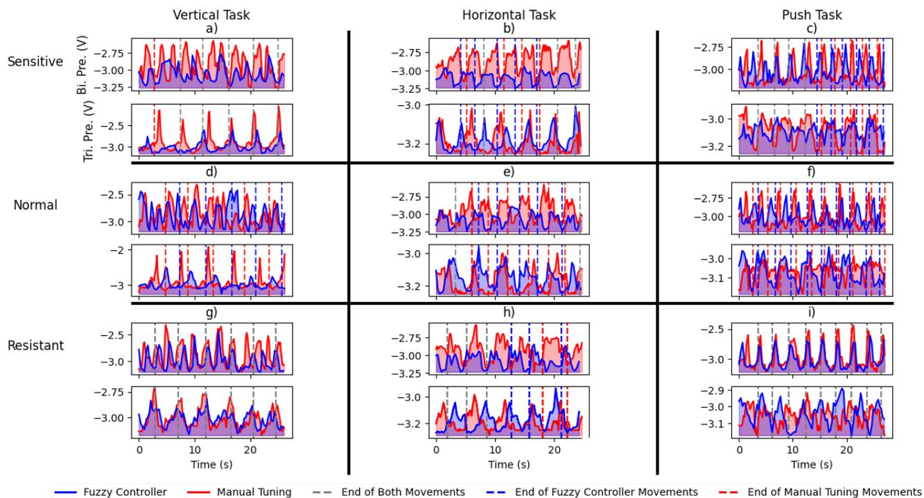
Fig. 5: Recorded pressure sensors signals for the sensitive (top row), normal (middle row), and resistant scenarios (bottom row). The plots correspond to the vertical (left column), horizontal (middle column), and pushing tasks (right column). In each task, the joint angle trajectory is plotted. The vertical dashed lines indicate when one trial of each task was completed and the next one started.
