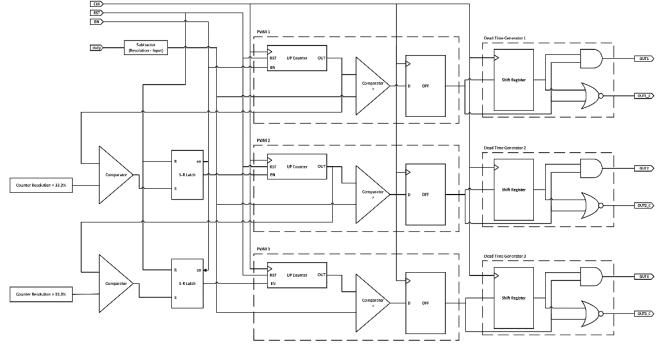
Figure 1 : Three phase PWM generator block diagram
