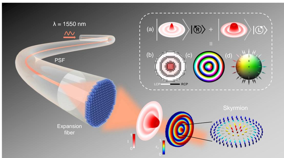
Fig. 1 The schematic diagram of the skyrmions' excitation from metafiber. The intensity and stokes vector distribution of the excitation light are shown (The vector of one whole skyrmion is detailed). Insert box: (a) The construction principle of skyrmion, composed by zero-order BB and first-order BB under orthogonal circular polarizations. The properties of the excited skyrmion including (b) polarization distribution and (c) spin distribution with (d) a HL-colored Poincaré sphere.
