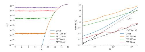
FIGURE 1. Left: The probability density function  $p(y) = \overline{f}^{\otimes 16}(y)$  for direct convolution and FFT-based convolution for the rareevent problem studied in Section 4.1. Right: The runtime for direct convolution and FFT-based convolution for the rare-event problem studied in Section 4.1.
