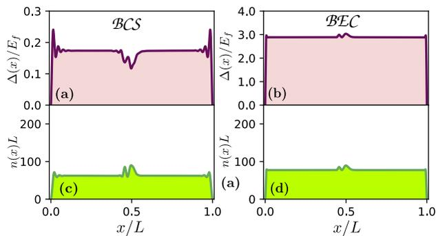
FIG. S2. Profiles of the gap function (top row) and density (bottom row) of a Fermi superfluid in the BCS regime with  $g = 1.0$  and  $\mu = 0.52E_f$  (left column) and BEC regime with  $g = 4.1$  and  $\mu = -0.07E_f$  (right column). The Rydberg potential stems from the Sr(71S) Rydberg state and its furthest dip is located at  $R_0 = L/2$ .
