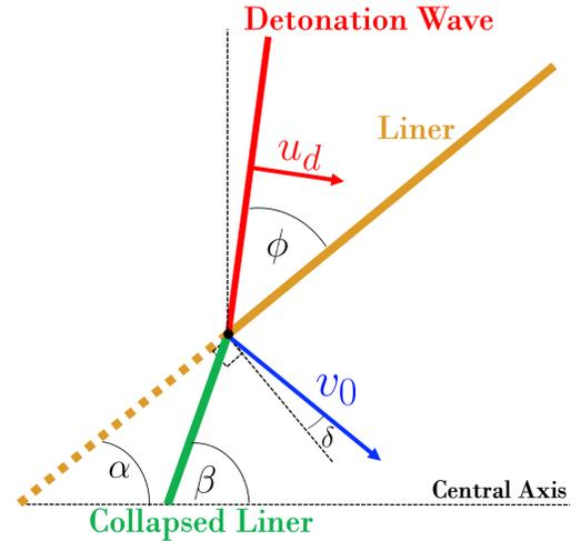
FIG. 1: This diagram shows the collapse of the liner from an initial angle  $\alpha$  to the collapse angle  $\beta$  as it is struck by a detonation wave moving with velocity  $u_d$  and at an angle  $\phi$  relative to the initial configuration of the liner. Each section of the liner collapses with a velocity  $v_0$  as the detonation wave sweeps along the liner. Reproduced from Sterbentz et al.<sup>24</sup>, with the permission of AIP Publishing.
