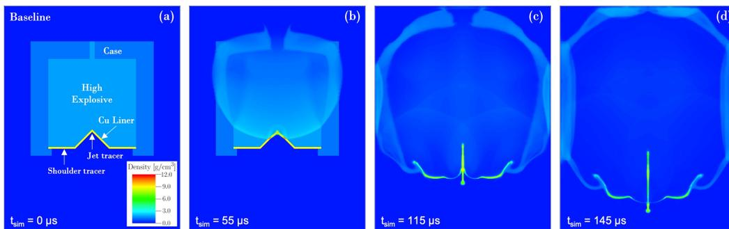
FIG. 4: 3D simulation images at several time instants for the baseline case, where the initial detonation occurs at time  $t = 0 \mu\text{s}$ : (a)  $t < 0 \mu\text{s}$ ; (b)  $t = 6 \mu\text{s}$ ; (c)  $t = 12 \mu\text{s}$ ; (d)  $t = 15 \mu\text{s}$ .
