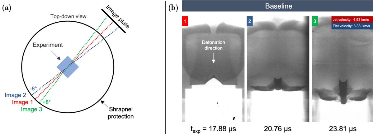
FIG. 7: (a) Experiment layout and (b) experimental radiographs for the baseline design. The orientation of the image source/plate to the experiment is  $0^\circ$ ,  $-8^\circ$ , and  $+8^\circ$  from left to right. Note that the spots in image 1 are from a damaged imaging plate.
