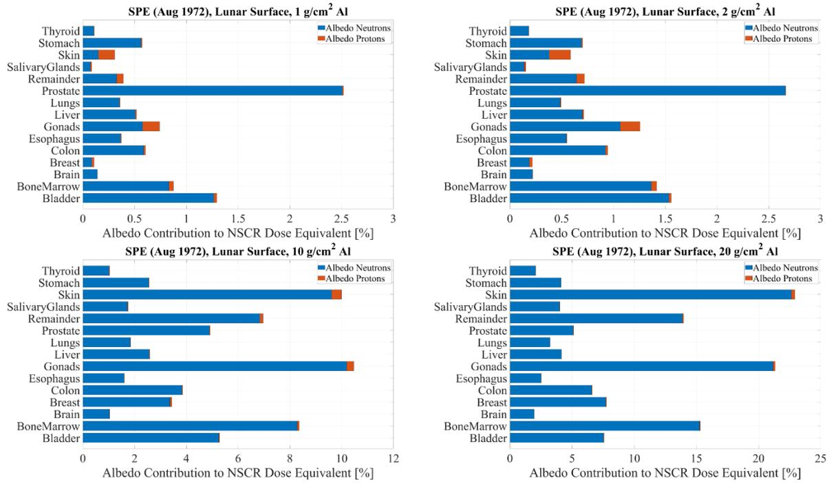
**Fig. 6.** Contribution of albedo neutrons and albedo protons to the NSCR dose equivalent behind various aluminum shielding thicknesses for SPE in August 1972 on the lunar surface.
