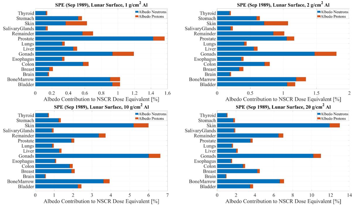
**Fig. 8.** Contribution of albedo neutrons and albedo protons to the NSCR dose equivalent behind various aluminum shielding thicknesses for SPE in September 1989 on the lunar surface.
