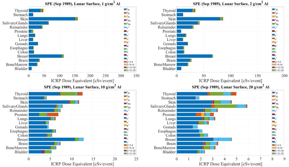
**Fig. 5.** Organ dose equivalent behind aluminum shielding with thicknesses of 1, 2, 10, and 20 g/cm<sup>2</sup> for SPE in September 1989 on the lunar surface, assessed with the ICRP model.
