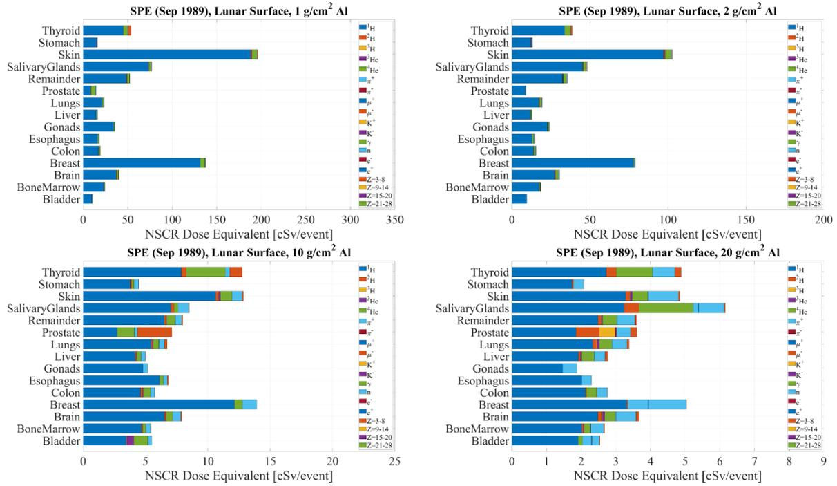
**Fig. 4.** Organ dose equivalent behind aluminum shielding with thicknesses of 1, 2, 10, and 20 g/cm<sup>2</sup> for SPE in September 1989 on the lunar surface, assessed with the NSCR model.
