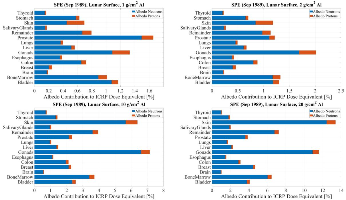
**Fig. 9.** Contribution of albedo neutrons and albedo protons to the ICRP dose equivalent behind various aluminum shielding thicknesses for SPE in September 1989 on the lunar surface.
