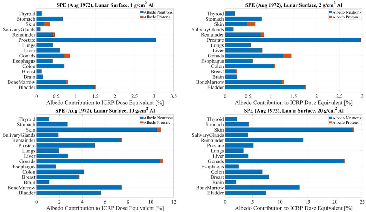
**Fig. 7.** Contribution of albedo neutrons and albedo protons to the ICRP dose equivalent behind various aluminum shielding thicknesses for SPE in August 1972 on the lunar surface.
