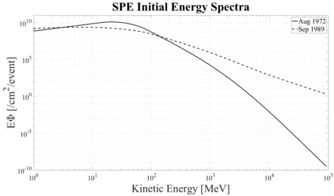
**Fig. 1.** Initial proton spectra generated in simulations to reconstruct SPEs in August 1972 and September 1989.
