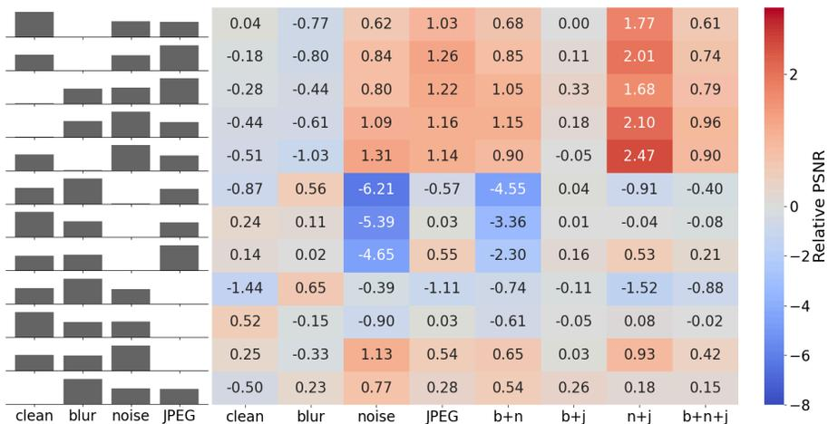
**Fig. 7:** Experimental results of different degradation distributions on Urban100. On the left side is the degradation distribution during training. The resulting performance on the respective degraded test set is on the right side (relative to uniform distribution).
