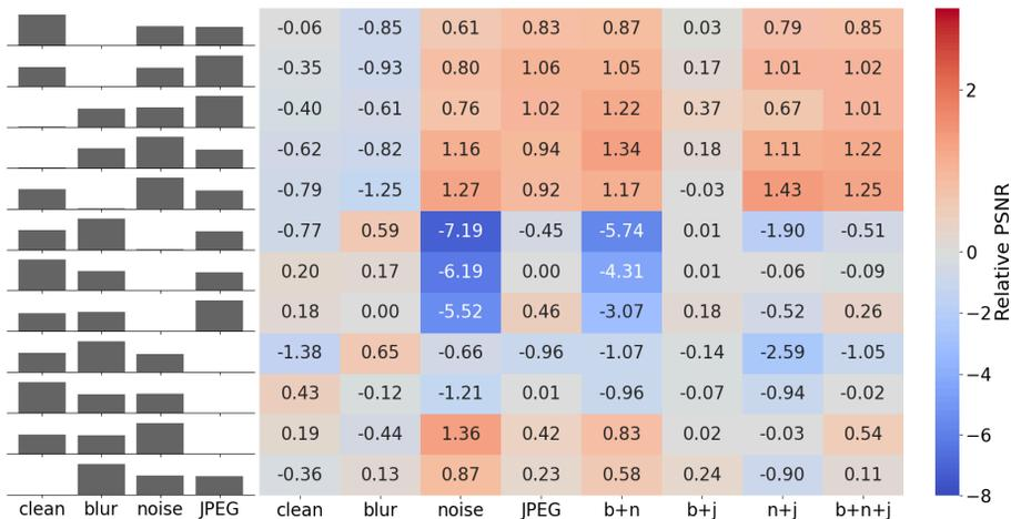
**Fig. 6:** Experimental results of different degradation distributions on Set14. On the left side is the degradation distribution during training. The resulting performance on the respective degraded test set is on the right side (relative to uniform distribution).
