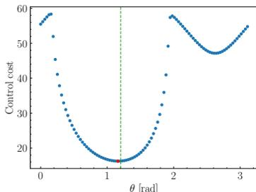
Fig. 6: The required control energy  $W_{\text{opt}}(\theta)$  of the optimal input for the Wasserstein terminal cost problem in (24). The green line and the red dot represent  $\theta_{\text{GW}}$  and  $\theta^*$ , respectively.
