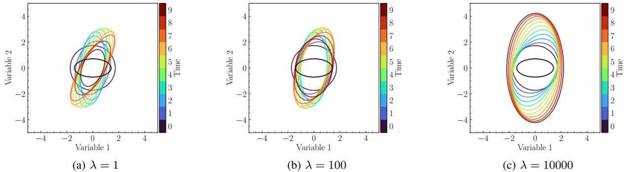
Fig. 4: The snapshots of the covariance matrices under the optimized policy for different values of  $\lambda$ . The colored lines indicate the  $2\sigma$  range of  $\Sigma_k$ , while the black line represents  $\Sigma_r$  in (22).
