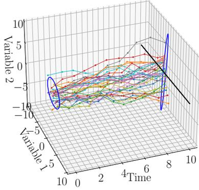
Fig. 3: One hundred sample paths of the systems controlled by the optimal policy for  $\lambda = 1$ . The blue circle denotes  $2\sigma$  range of  $\Sigma_0$  and  $\Sigma_N$  and the black line denotes the degenerated target distribution  $\Sigma_r$  in (21).
