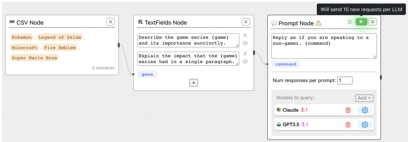
**Figure 3: An example of chaining prompt templates, one of ChainForge’s unique features. Users can test different templates at once by using the same input variable (in {} brackets). Templates can be chained at arbitrary depth using TextFields nodes. The user is hovering over the Run button of the Prompt Node, displaying a reactive tooltip of how many queries will be sent off.**
