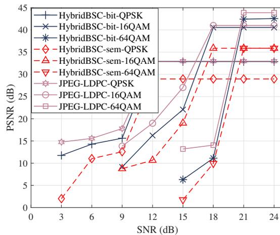
Fig. 3: The PSNR score versus SNR in Rayleigh channel.
