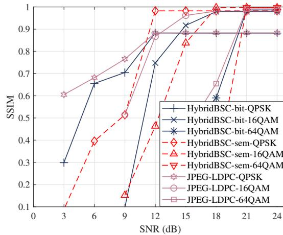
Fig. 5: The SSIM score versus SNR in Rayleigh channel.
