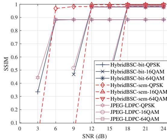
Fig. 4: The SSIM score versus SNR in AWGN channel.
