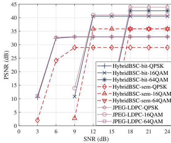
Fig. 2: The PSNR score versus SNR in AWGN channel.
