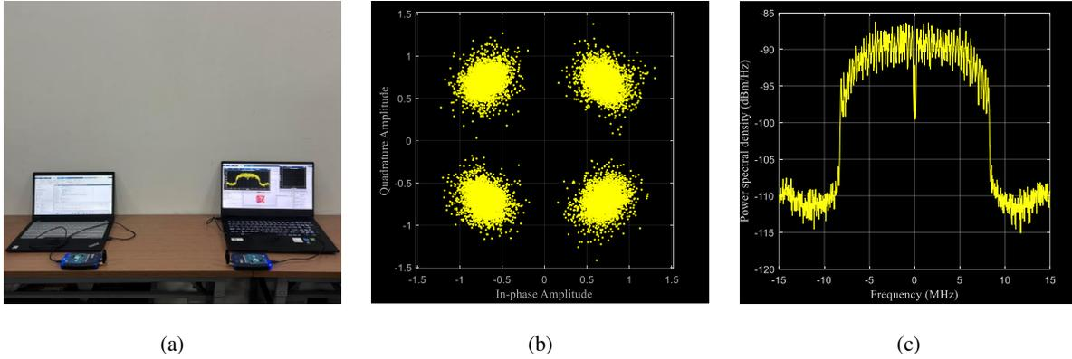
Fig. 6: The pluto-based SDR wireless HybridBSC prototype. (a) Real experimental scenario of the proposed HybridBSC in a indoor LoS environment; (b) Example of I/Q signals transmitted with QPSK modulation. (c) Example of received baseband WLAN signal spectrum in the wireless testbed.
