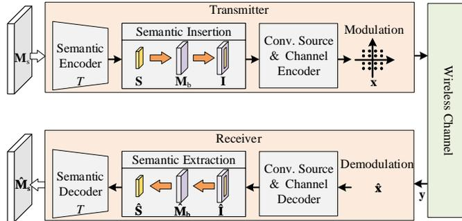
Fig. 1: The structure of the proposed HybridBSC.
