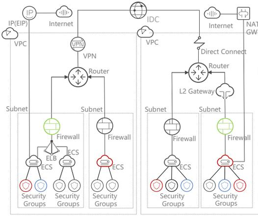
Fig. 1: Example of the most common VPC services and their interconnect
