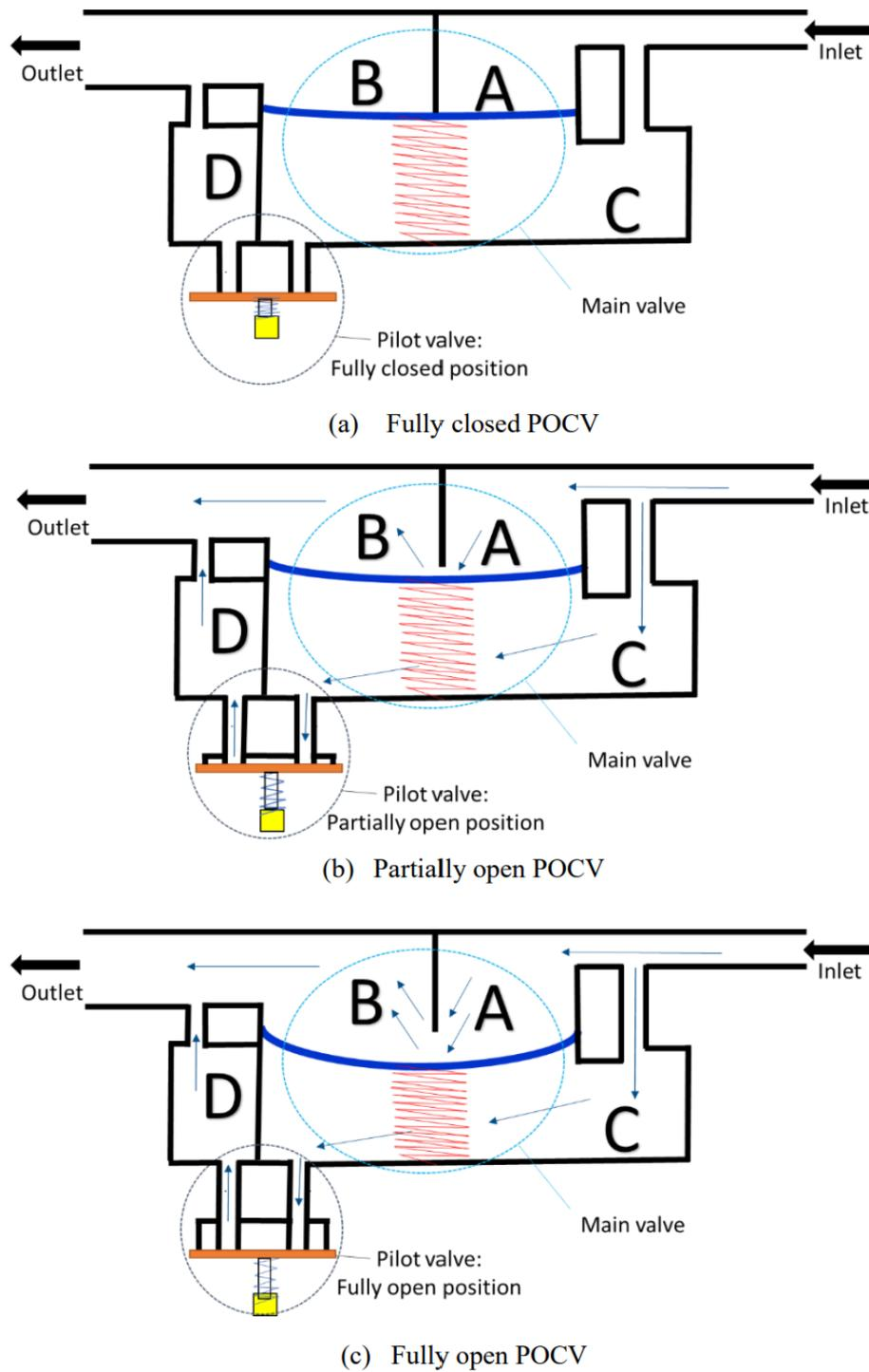
Figure 2: Schematic views of the pilot-operated valve under investigation for different opening setpoints. The valve can be operated as ON/OFF valve ((a) → (c)), and is designed to work as a proportional valve ((a) → (b) → (c)). A: Inflow region; B: Outflow region; C: Pilot chamber region; D: Pilot chamber outflow.
