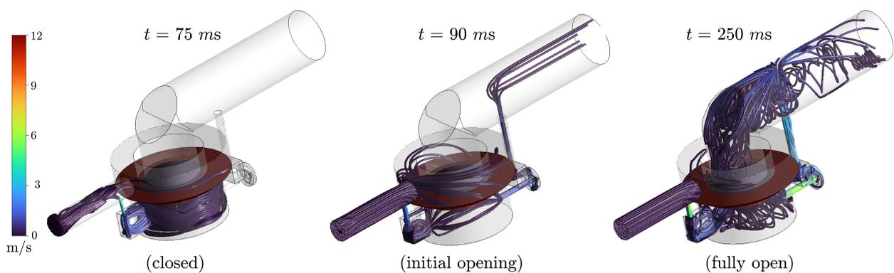
Figure 15: Streamlines during opening of the POCV according to Figure 13 at  $t = 75$  ms (left),  $t = 90$  ms (center) and  $t = 250$  ms (right) at differential pressure 0.5 bar.
