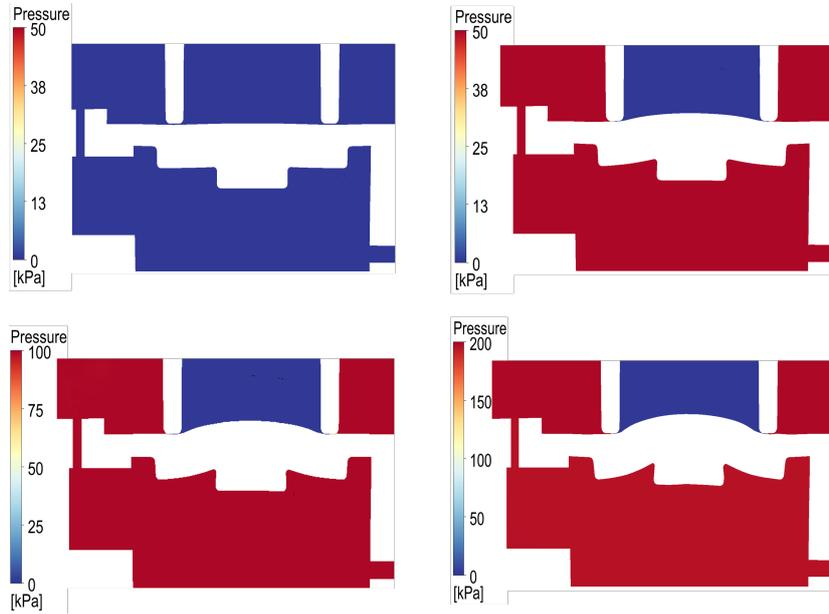
Figure 7: Plane section view of the normally closed POCV at 0 bar (*top left*), 0.5 bar (*top right*), 1 bar (*bottom left*) and 2 bar (*bottom right*). Colors indicate pressure distribution.
