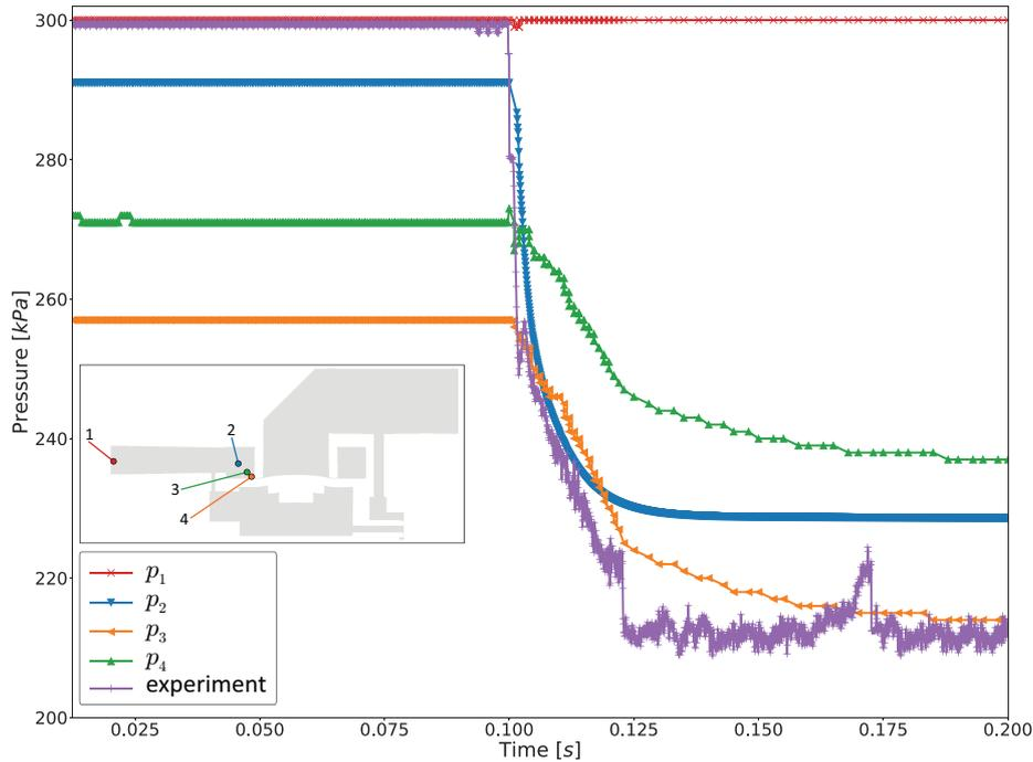
Figure 11: Pressure evolution during opening of the POCV at differential pressure 3 bar: Computed pressure at 3 points near the valve-seat gap and at the inlet, and experimental data.
