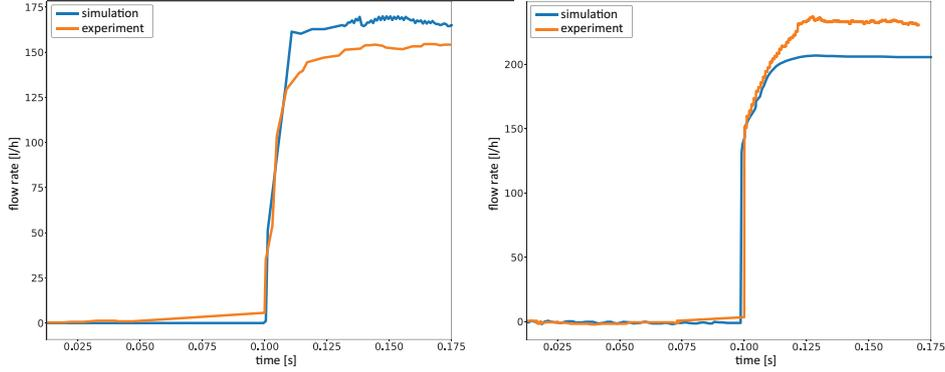
Figure 12: Computed flow rate and experimentally obtained flow rate for a differential pressure of 2 bar (*left*) and 3 bar (*right*).
