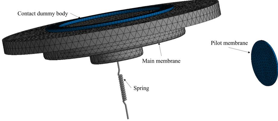
Figure 4: POCV structural system after spatial discretization. The main membrane is constrained by a contact dummy body representing the valve seat and a spring to guide the deformation. The pilot membrane is clamped and controlled by a displacement boundary condition to replicate the SMA-based actuator actions.
