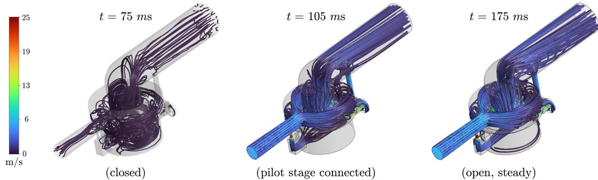
Figure 10: Streamlines during the opening of the microfluidic POCV at  $t = 75$  ms (*left*),  $t = 105$  ms (*center*) and  $t = 175$  ms (*right*) for an inlet pressure of 3 bar.
