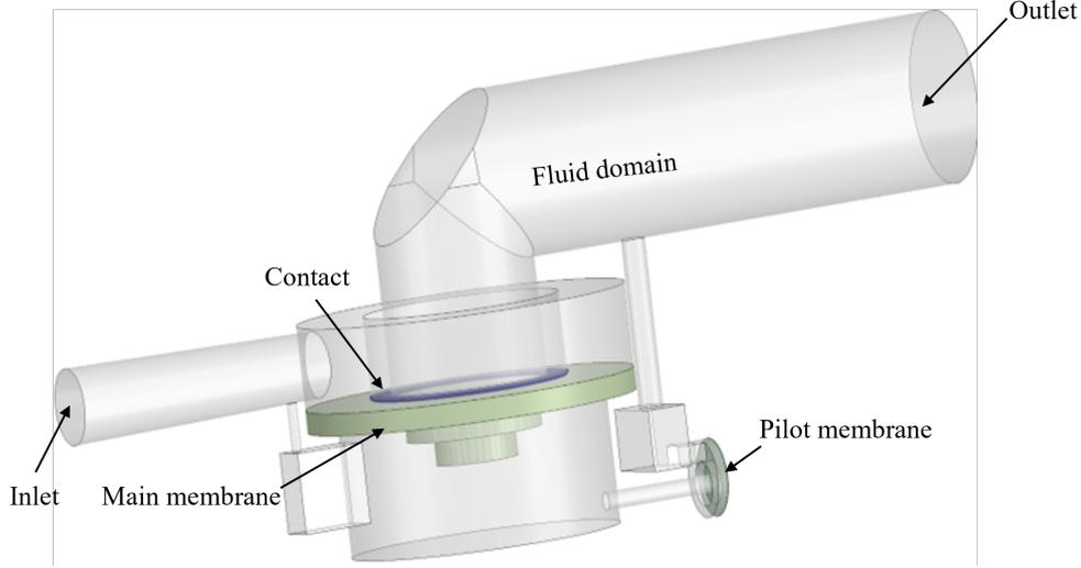
Figure 3: Illustration of the pilot-operated control valve.
