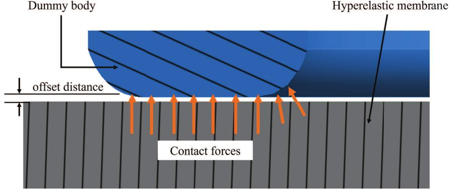
Figure 5: Membrane to valve seat inter-body contact modelling. Blue: Contact dummy body section. Grey: Main membrane section. The mechanical parts are separated by a thin gap of thickness  $\epsilon > 0$  equal to the fluid gap width for consistency.
