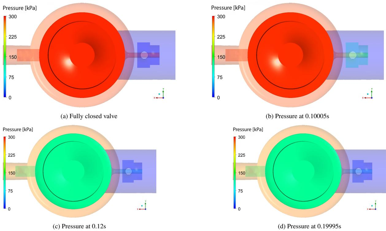
Figure 9: Pressure contour snapshots of the POCV. The top right panel shows the pressure drop at the vicinity of the pilot membrane shortly after opening actuation, the bottom left and right panels display the pressure at different times corresponding to a fully open valve. Note the valve's fast time-to-open response from 3 bar to 1.7 bar (around 20 ms).
