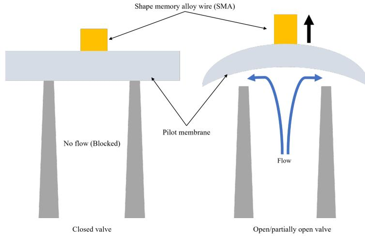
Figure 1: Illustration of the actuation control based on shape memory alloy material (Yellow). The left-hand side corresponds to a closed POCV; the pilot membrane (Silver) is undeformed, and the upstream flow is blocked. The right-hand side corresponds to an actuated valve; the pilot membrane deforms according to the current SMA position, and the POCV switches to a partially or fully open position.
