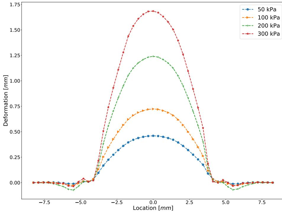
Figure 8: Membrane deflection of the normally closed valve for inlet pressure values  $p_{in} \in \{0.5, 1, 2, 3\}$  bar.
