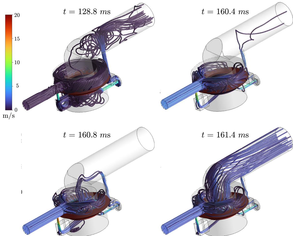
Figure 17: Streamlines during attempted proportional operation of the POCV at a differential pressure of 1 bar at  $t = 128.8 \text{ ms}$  (top-left),  $t = 160.4 \text{ ms}$  (top-right),  $t = 160.8 \text{ ms}$  (bottom-left) and  $t = 161.4 \text{ ms}$  (bottom-right).
