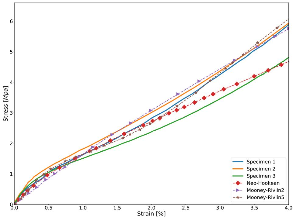
Figure A.18: Curve-fitting results of the Hyperelastic material calibration. Stress versus strain curve plots for experimental data versus different hyperelastic material models. Red: Curve fitting using the neo-Hookean model. Violet: Curve fitting using the Mooney-Rivlin model with 2 parameters material model. Cyan: Curve fitting using the Mooney-Rivlin model with 5 parameters material model. Black: Experimental results.
