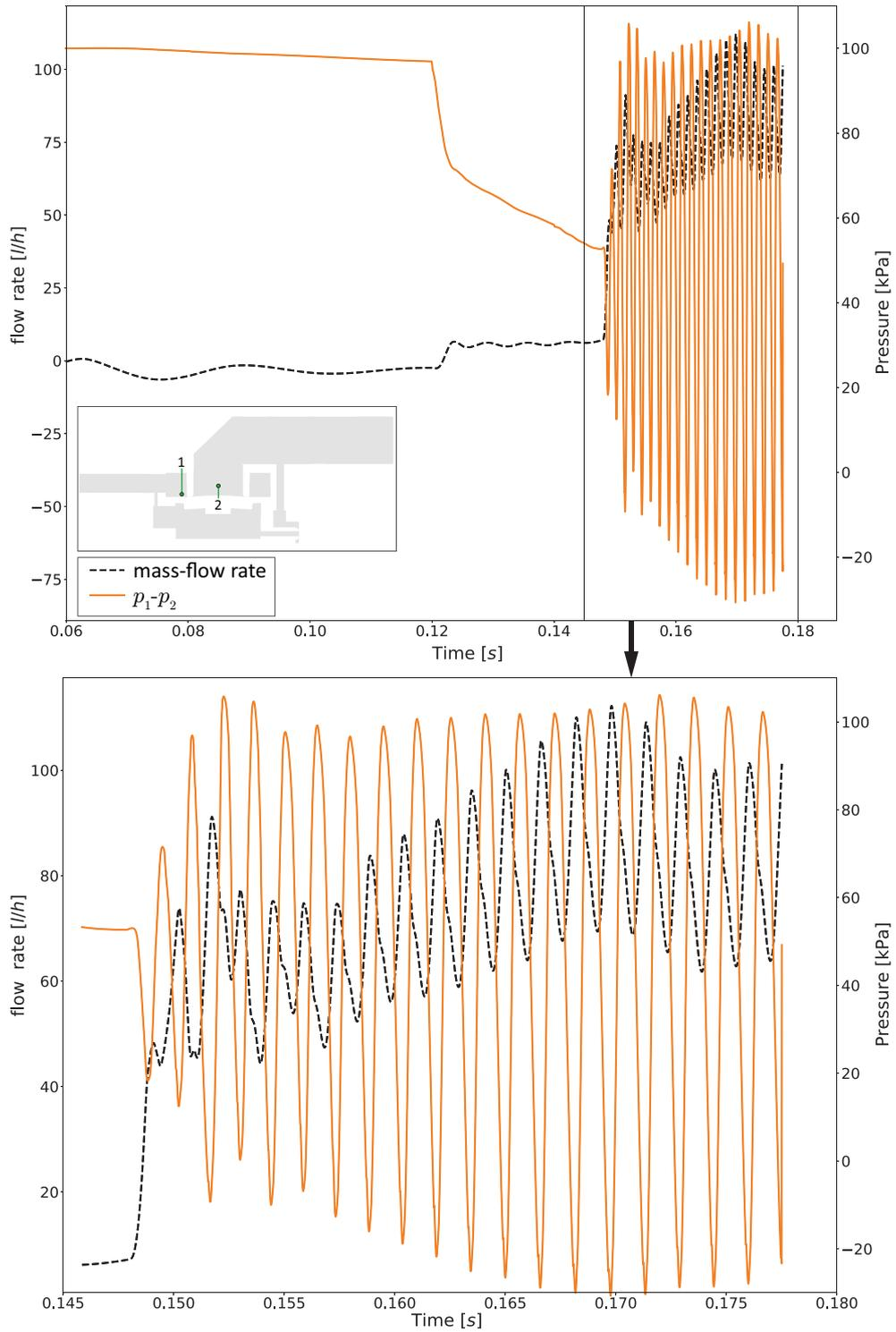
Figure 16: Evolution of the flow rate and upstream-downstream pressure difference during proportional operation of the POCV for an inlet pressure of 1 bar.
