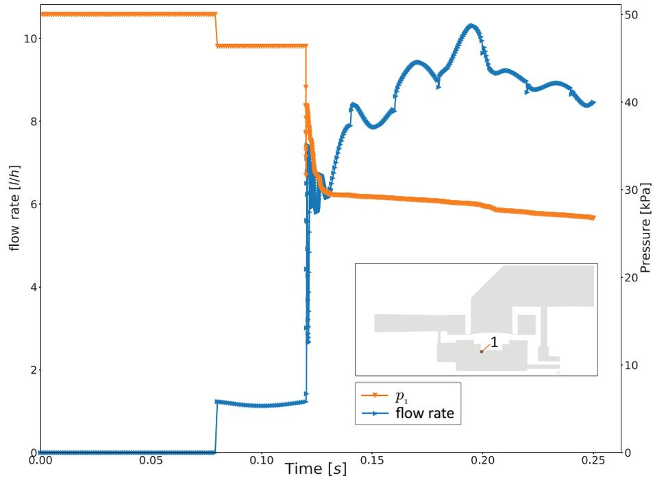
Figure 14: Flow-rate and pressure evolution during the opening of the POCV in accordance with Figure 13 at differential pressure 0.5bar.
