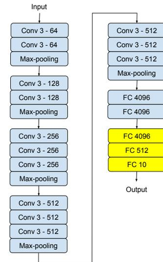
Figure 5: Diagram of the VGG-16 model for training on CIFAR-10 dataset. ‘‘Conv {receptive field size} - {number of output channels}’’ depicts the convolutional layers. ‘‘FC {output size}’’ depicts the fully connected layers.
