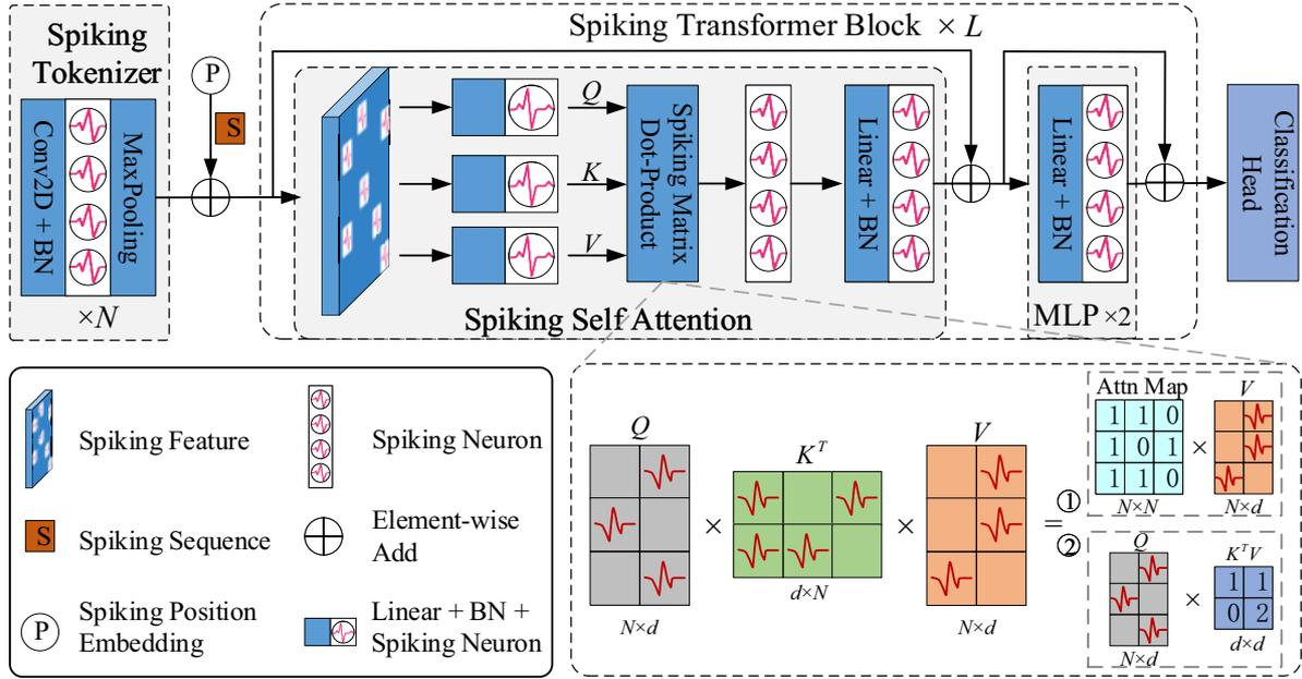
**Figure 1.** The overview of Spiking Transformer (Spikformer).
