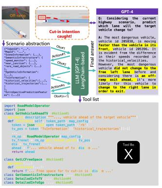
Fig. 10: Demonstration of highway scenario processing using the LangChain-based pipeline with GPT-4. GPT-4 initiates with the 'GetVehicleAheadTV' tool and receives an observation indicating the presence of a small vehicle ahead of the target vehicle (TV). Following further inferences, the model ultimately predicts the cut-in intention of the target vehicle in advance. Further, the explanations provided by the model are similar to human thought processes.
