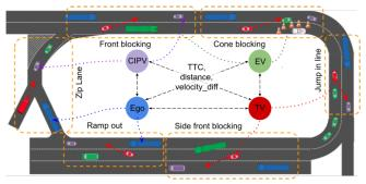
Fig. 5: ESP Token Types - Representation of Ego (Ego vehicle), CIPV (Vehicle in front of ego), EV (Environmental vehicle), and TV (Target vehicle) within each time frame. Scenario types are determined based on rule-based criteria.
