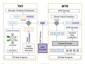
Fig. 4: Seamless Integration of ESP Features with Motion Prediction Models. The ESP plugin seamlessly integrates with widely used encoder-decoder models such as TNT and MTR. As depicted, ESP enhances existing features through straightforward concatenation, leading to a transformative advancement in motion prediction.
