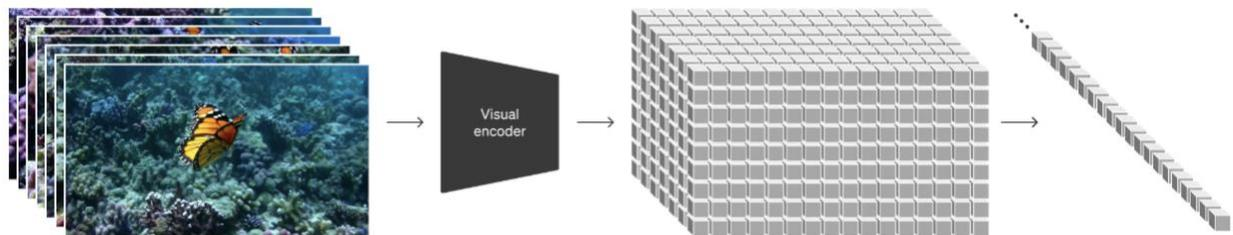
**Figure 1** Process of converting videos to lower dimensions and dividing them into patches
