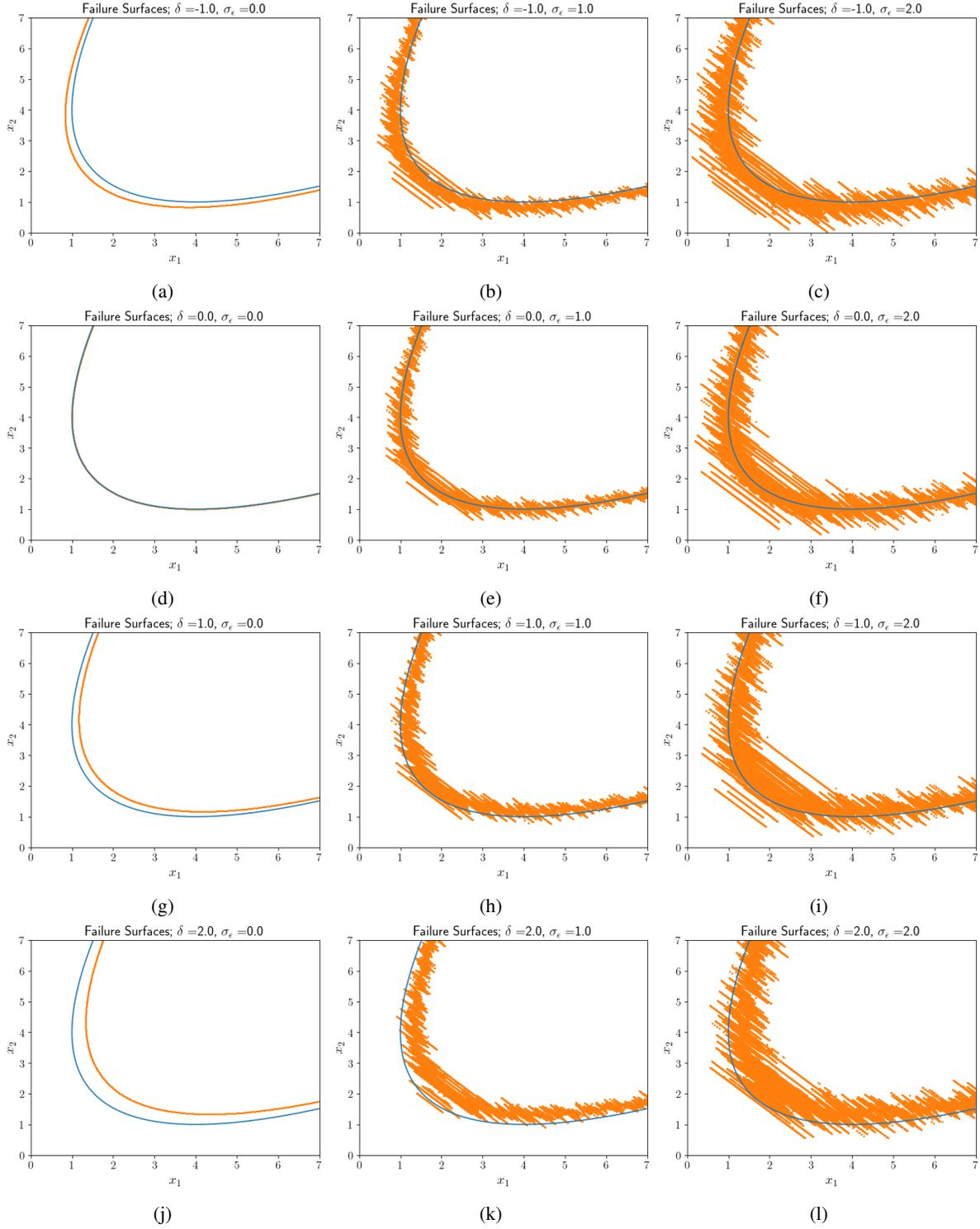
Figure 2: Example 1: Failure limit surface comparisons. In each figure, the solid blue line corresponds to  $H(\mathbf{x}) = 0$ , while the orange dashed line corresponds to  $L(\mathbf{x}) = 0$ . The title of each subfigure shows the values of  $\delta$  and  $\sigma_\epsilon$ .
