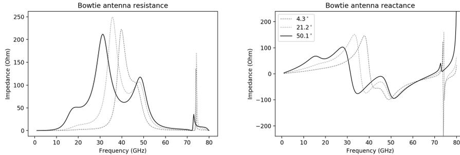
**Figure 3.** The simulated resistance and reactance of the bowtie antenna, calculated using Ansys HFSS. The simulation shows that the antenna reactance diminishes as the flare angle increases and the first resonance widens. The solid line, labeled with a flare angle of  $50^\circ$ , is the nominal configuration. We drive this antenna at  $100\Omega$  using a quasi-CPW line in our design.
