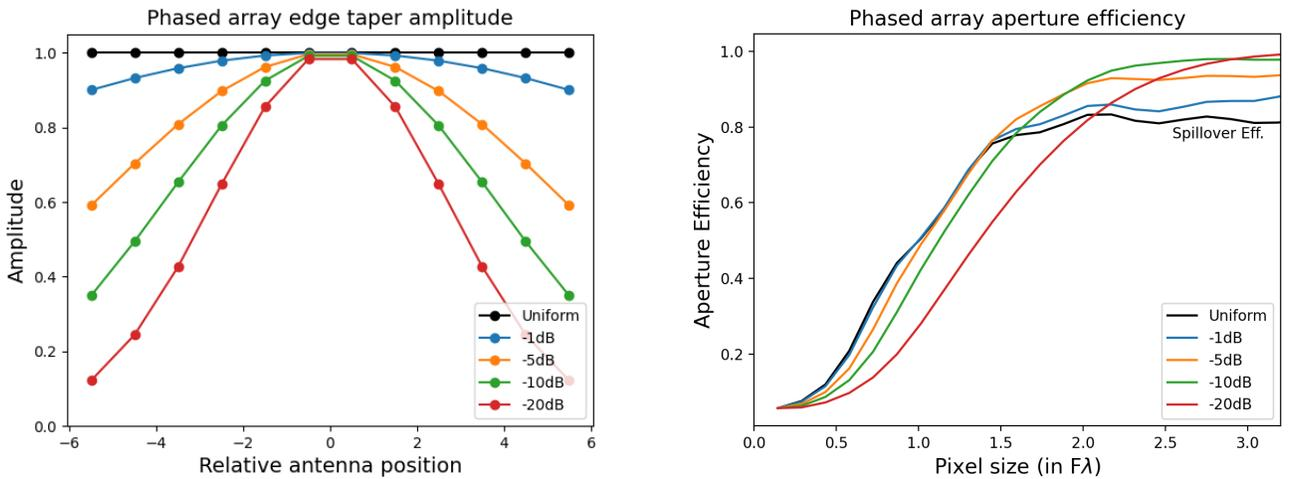
**Figure 13.** (Left) Illumination of an example 12-element antenna array with different edge tapers. (Right) Calculation of the aperture efficiency of a  $N \times N$  antenna array with different edge tapers. The dashed lines show a uniformly illuminated array's illumination and spillover efficiencies. The antenna array presented in this publication is uniformly illuminated with a pixel size of  $\sim 1.5, 2.0F\lambda$  for the two bands, respectively.
