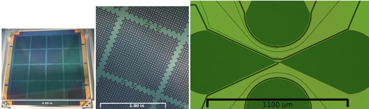
**Figure 2.** Bowtie tile. (a) Photograph of a full tile showing a 4x4 grid of pixels. (b) Zoom in on a pixel. We have a 12x12 pairs of bowtie antennas comprising the antenna array with four bolometers capturing A/B polarization at our two bands. (c) Zoom in on a single antenna element. Dark green indicates the ground plane cutout showing both the sub-antenna and the co-planar waveguide driving the antenna.
