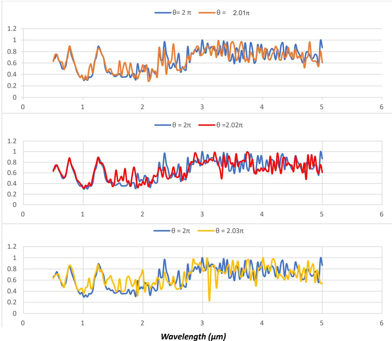
**Fig 11.** The effects of increasing the  $\theta$  parameter of the Archimedean spiral ( $r = a + b*\theta$ ) on the absorption spectrum of the metamaterial absorber
