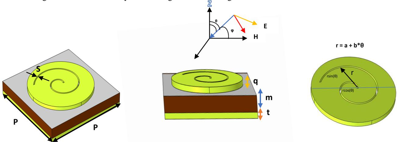
**Fig 1.** The proposed metamaterial absorbent structure has a size ( $p$ ) of  $2.5 \mu\text{m}$ . This design consists of three layers, the metal layers of gold with thicknesses of  $t = 0.1 \mu\text{m}$  and  $q = 0.1 \mu\text{m}$  and the middle layer of vanadium oxide with a thickness of  $m = 0.27 \mu\text{m}$  and the size of the Archimedes spiral  $s = 0.04 \mu\text{m}$ .
