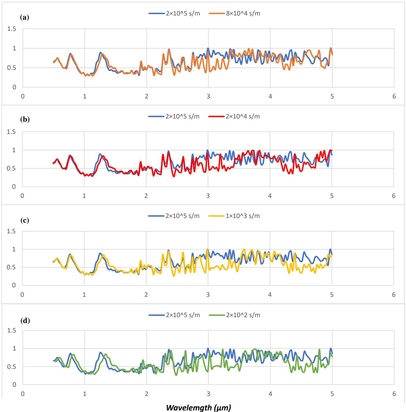
**Fig 2.** Analysis of the TE wave absorption spectrum of vanadium oxide (VO<sub>2</sub>) under different conductivity conditions, which is compared with the absorption spectrum diagram in conductivity  $2 \times 10^5$  s/m, (a)  $8 \times 10^4$  s/m, (b)  $2 \times 10^4$  s/m, (c)  $1 \times 10^3$  s/m, (d)  $2 \times 10^2$  s/m.
