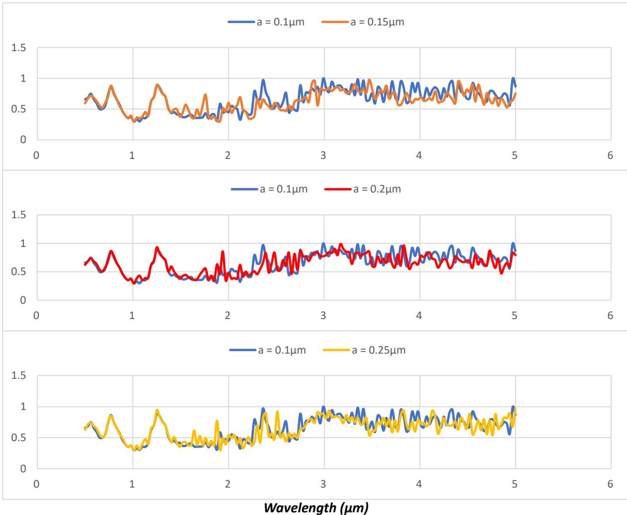
**Fig 12.** The effects of increasing the a parameter of the Archimedean spiral ( $r = a + b*\theta$ ) on the absorption spectrum of the metamaterial absorber
