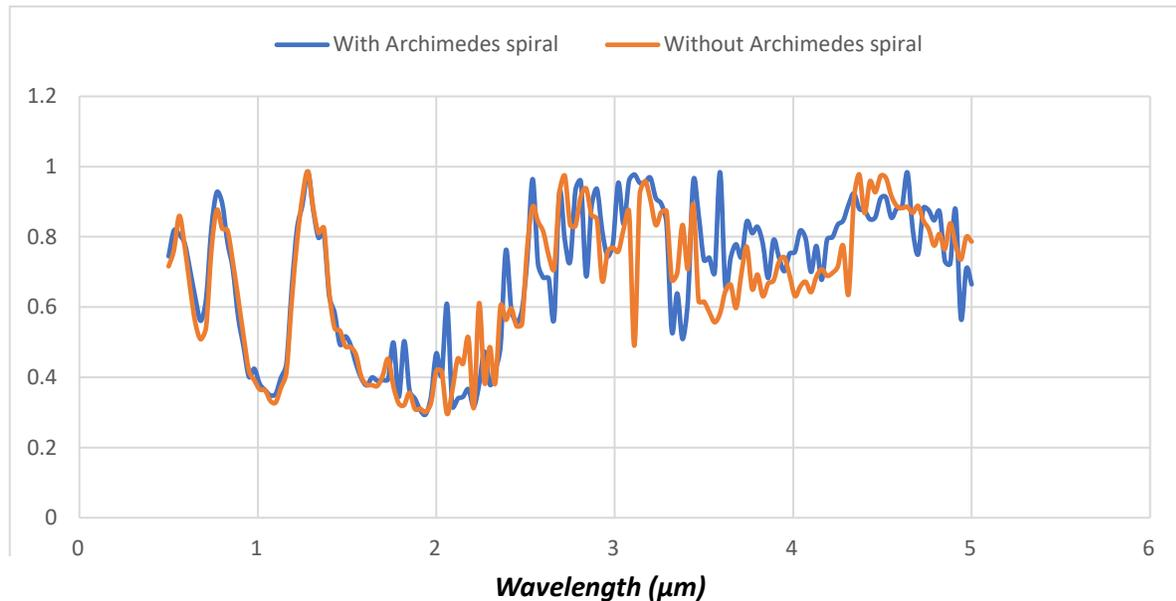
**Fig 6.** Comparison diagram of TM polarization absorption for metamaterial absorbent structure with and without Archimedean structure
