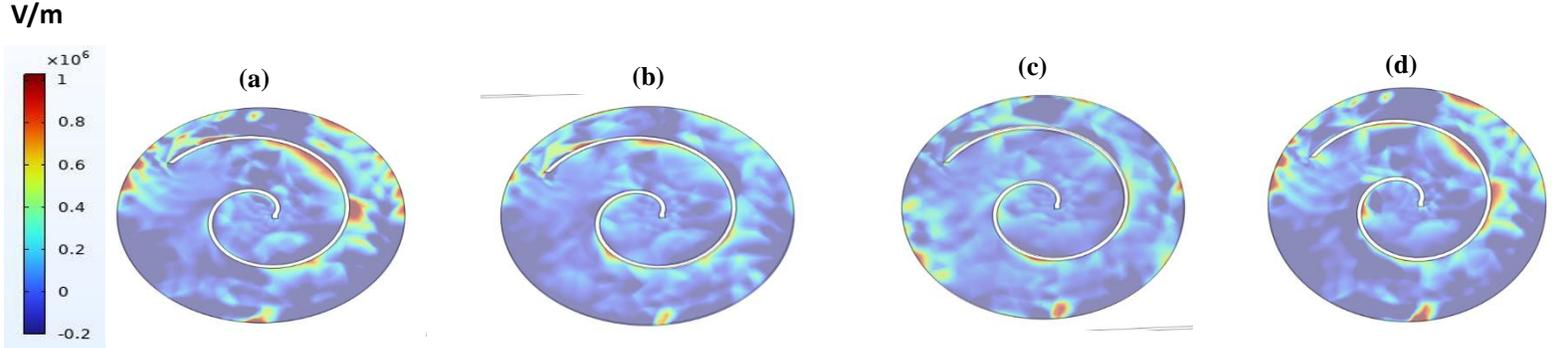
**Fig 3.** Z-component of electric field distribution on gold Archimedean spiral structure at  $\lambda = 2.99 \mu\text{m}$ , TE polarization,  $\theta = 45^\circ$  radiation angle, and  $\phi = 0^\circ$  for conductivity (a)  $8 \times 10^4$  s/m, (b)  $2 \times 10^4$  s/m, (c)  $1 \times 10^3$  s/m, (d)  $2 \times 10^2$  s/m.
