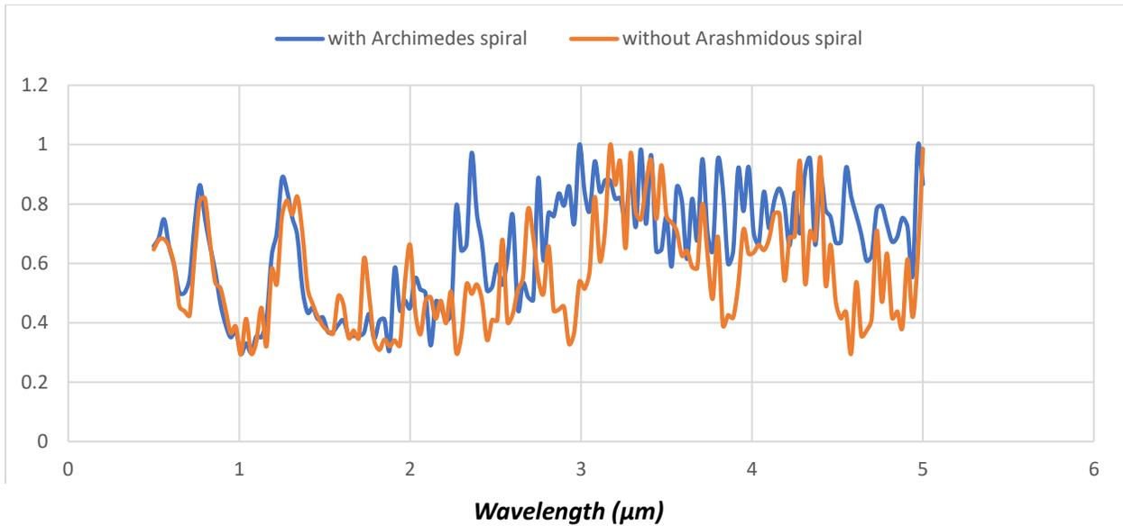
**Fig 4.** Comparison diagram of TE polarization absorption for metamaterial absorbent structure with and without Archimedean structure
