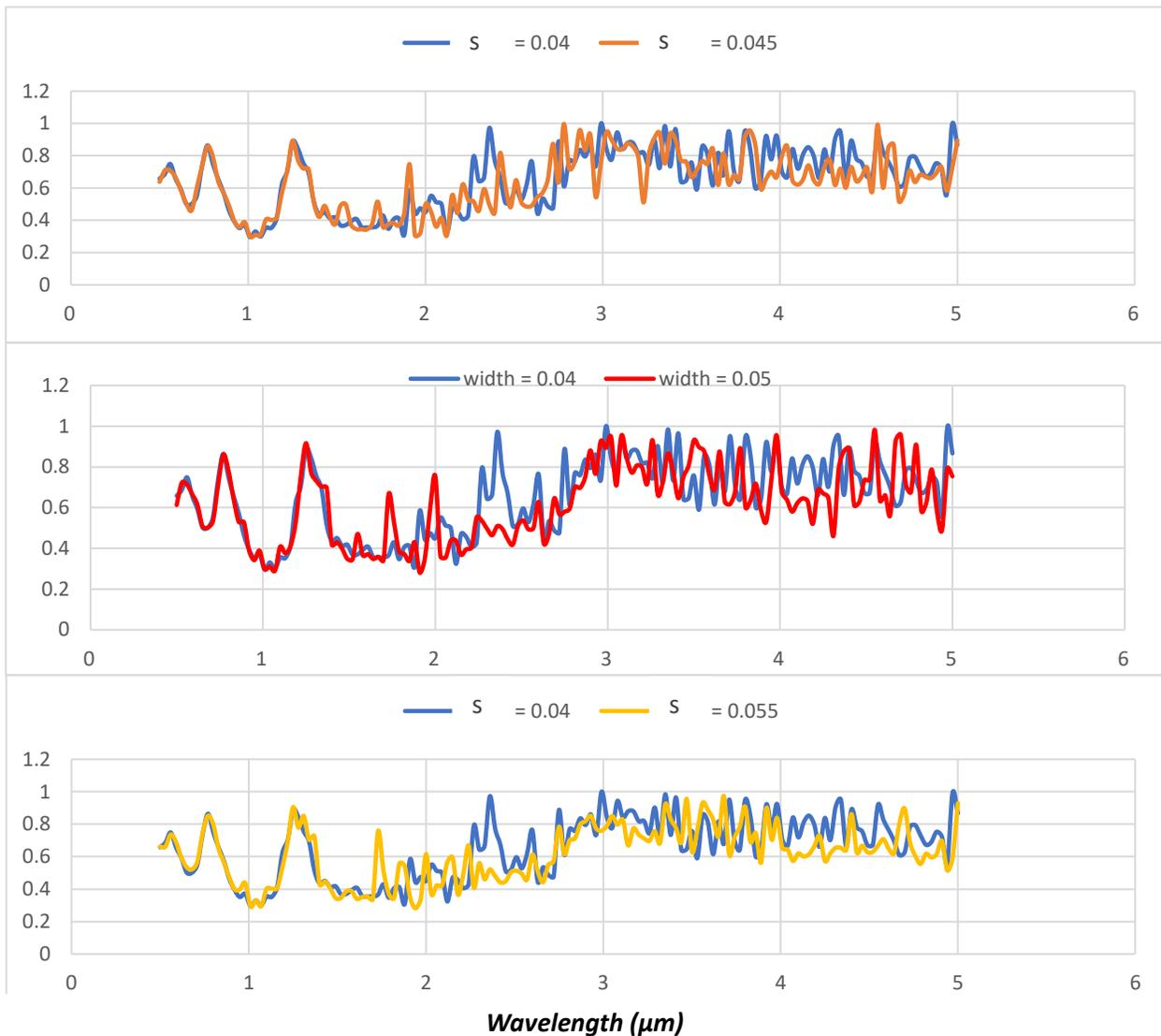
**Fig 10.** Investigating the effect of Archimedes screw thickness on absorption spectrum of metamaterial absorber
