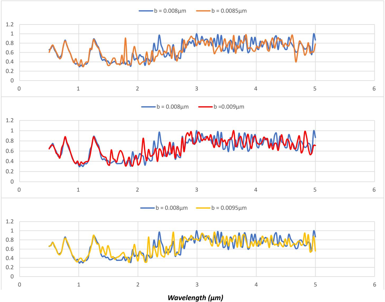
**Fig 12.** The effects of increasing the  $b$  parameter of the Archimedean spiral ( $r = a + b*\theta$ ) on the absorption spectrum of the metamaterial absorber
