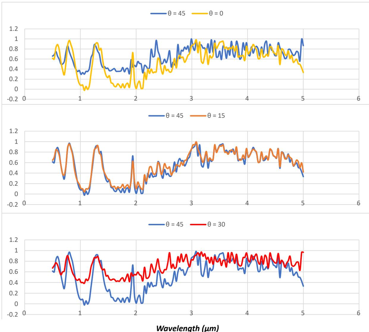
**Fig 9.** Absorption spectra of metamaterials at different azimuthal angle  $\theta$  for TE configuration ( $\varphi = 0^\circ$ , conductivity of vanadium oxide =  $2 \times 10^5$  s/m)
