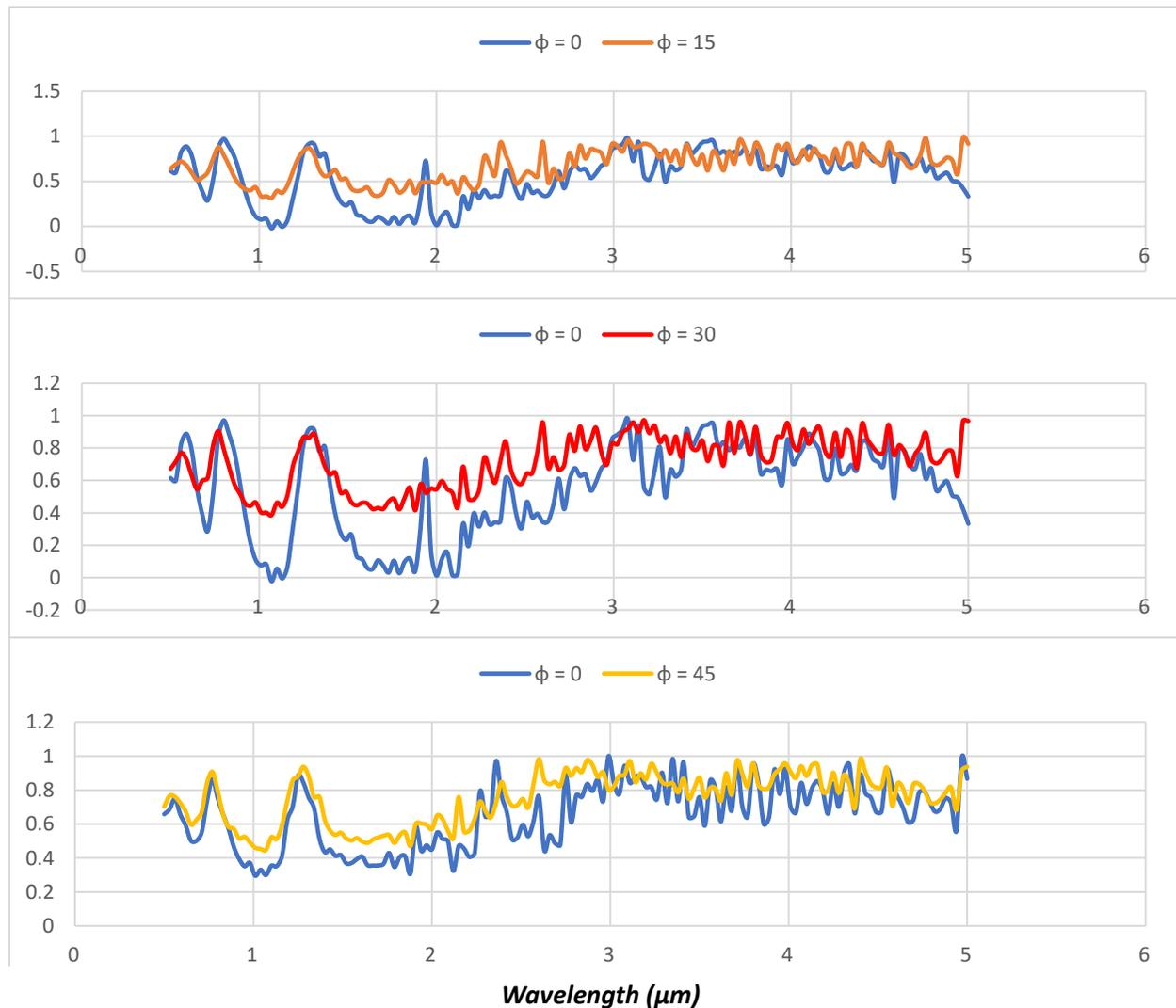
**Fig 8.** Absorption spectra of metamaterials at different azimuthal angle  $\varphi$  for TE configuration ( $\theta = 45^\circ$ , conductivity of vanadium oxide =  $2 \times 10^5$  s/m)
