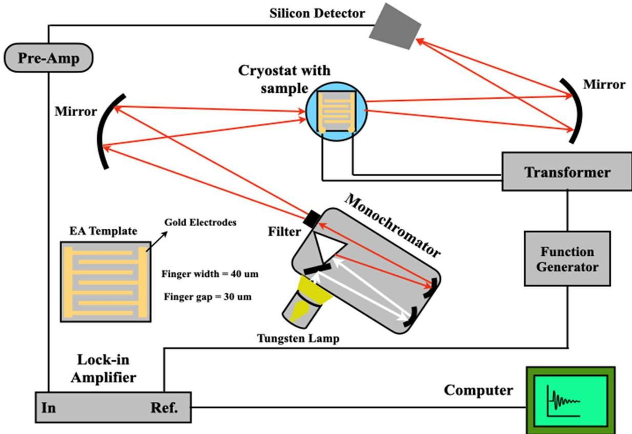
FIG. S1. The electroabsorption setup.
