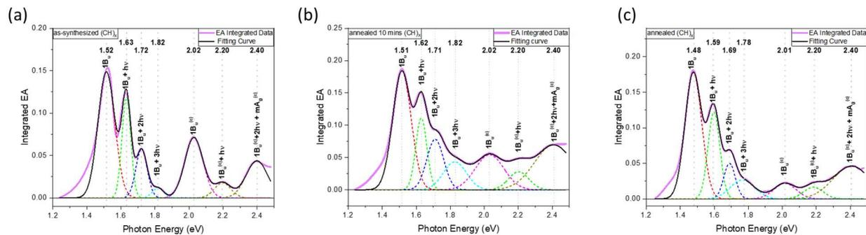
FIG. S5. Integrated EA spectra of as-synthesized, 10 and 30 min annealed  $(\text{CH})_x$  film.
