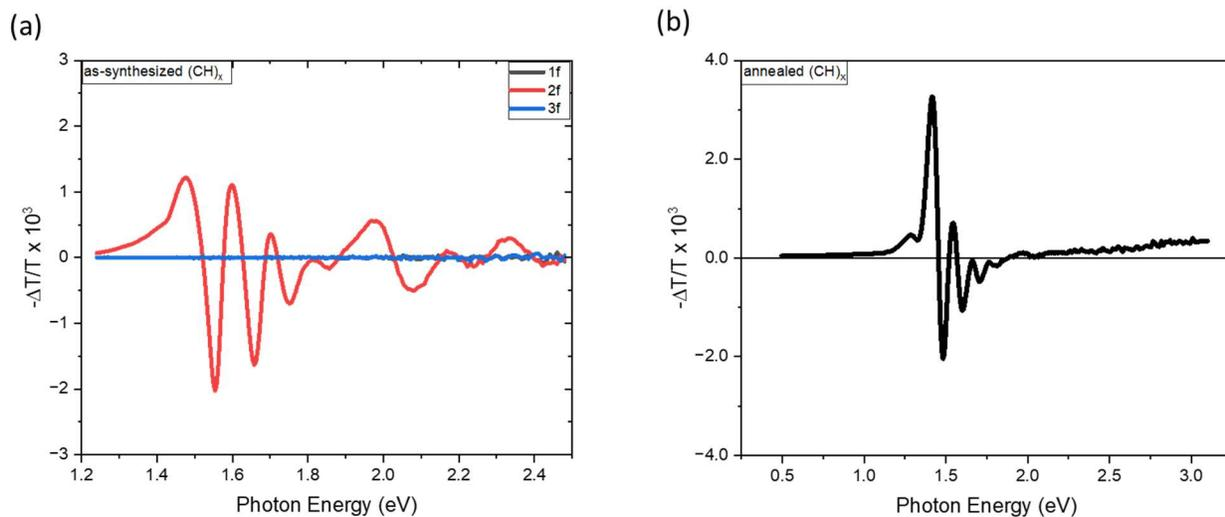
FIG. S2. (a) The electroabsorption spectra measured at  $1f$ ,  $2f$  and  $3f$  as indicated. (b) The EA spectrum for an annealed  $(\text{CH})_x$  film plotted in a broad spectral interval of 0.5 to 3 eV.
