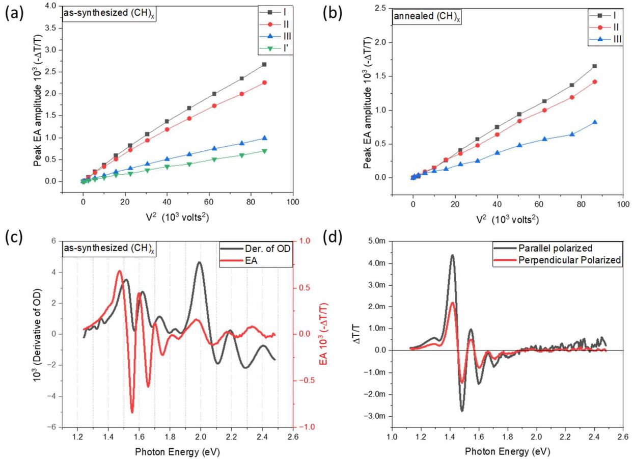
**FIG. 3.** The EA strengths vs  $V^2$  for the as-synthesized (a) and annealed (b)  $(CH)_x$  films at several photon energies that correspond to peaks in the EA spectra as denoted in Fig. 2(a). (c) Comparison between the EA spectrum and the derivative (Der) of the absorption spectrum for the as-synthesized  $(CH)_x$  film. (d) The EA spectra of a  $(CH)_x$  film measured at two different light polarization, namely, parallel (black) and perpendicular (red) to the applied electric field.
