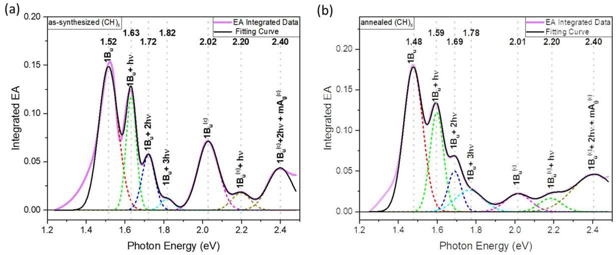
FIG. 4. The integrated EA spectra of (a) the as-synthesized and (b) the annealed  $(\text{CH})_x$  film. Various bands and phonon replica are assigned (see Table 1). The broken lines through the data are a fit using the Huang-Rhys model (Eq. (2)).
