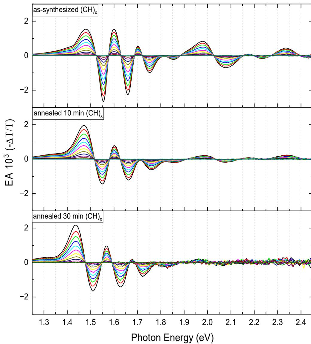
FIG. S4. The EA spectra for as-synthesized, and 10 and 30 min annealed  $(CH)_x$  films.
