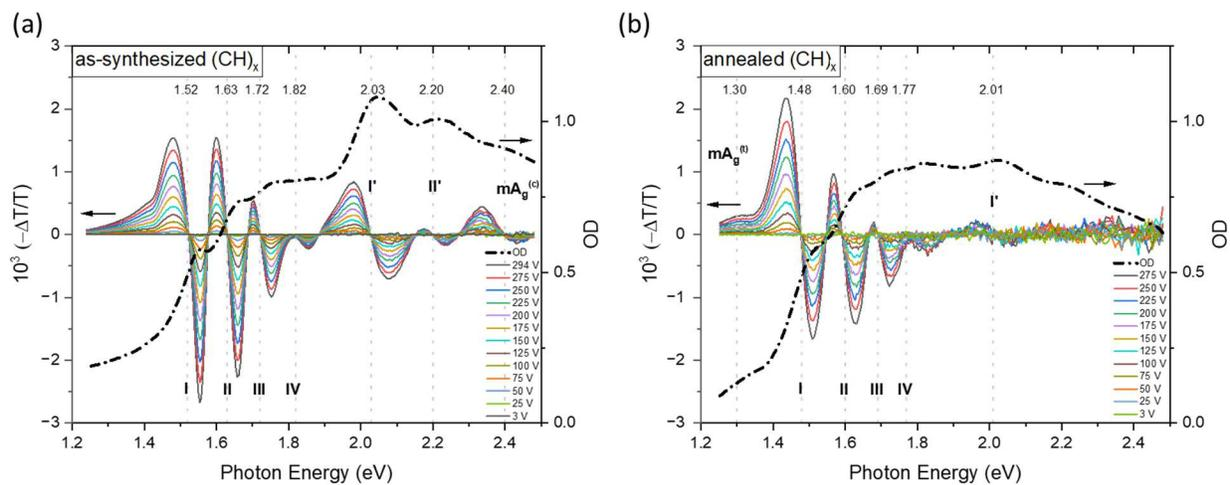
FIG. 2. The electroabsorption (EA) spectra for various applied voltages compared with the absorption spectra (OD) (•-•) for 'as synthesized' (a) and 'annealed' (b)  $(\text{CH})_x$  thin film. The zero-crossing photon energies, I-IV and the  $\text{mA}_g^{(t)}$  band are assigned for the *trans*- $(\text{CH})_x$  isomer; and I', II' and  $\text{mA}_g^{(c)}$  are assigned for the *cis*- $(\text{CH})_x$  isomer.
