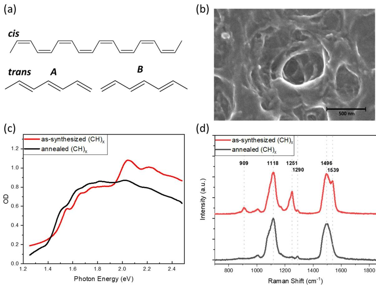
**FIG. 1.** (a) The *cis*- and *trans*-(CH)<sub>x</sub> structures and the two phases of the *trans*-(CH)<sub>x</sub> isomer are denoted. (b) SEM image of the fibrils in a (CH)<sub>x</sub> thin film. (c) The absorption spectrum of a (CH)<sub>x</sub> film before (red line) and after annealing (black line), plotted as optical density (OD). (d) Resonant Raman spectra of a (CH)<sub>x</sub> film before (red) and after annealing (black). Few Raman active vibrations are assigned.
