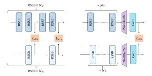
Figure 6. Left: The structure of mid-level feature distillation; Right: The structure of end-level feature distillation
