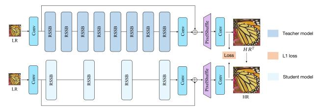
Figure 5. The deep feature distillation pipeline of our method.
