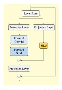
Figure 4. The structure of Vision Mamba Module(ViMM).
