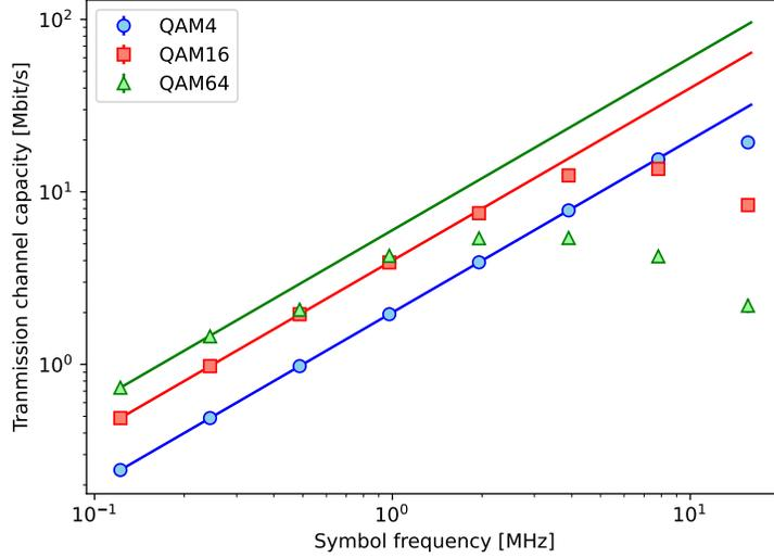
Fig. 10. Channel capacities for calculated SER for each of the measured modulation schemes as a function of symbol frequency. The continuous lines represent channel capacities in case of errorless communication.
