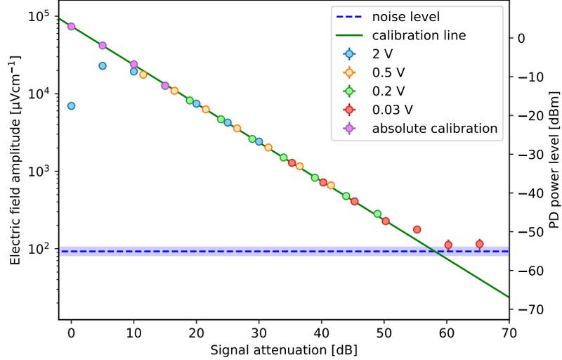
Fig. 5. Amplitude of the SIG field (left vertical axis) as the function of signal attenuation. The right vertical axis refers to the PD signal power level calculated from the Fourier power spectrum for heterodyne detection. The blue area around the shot noise level corresponds to the standard error of the calculated value.
