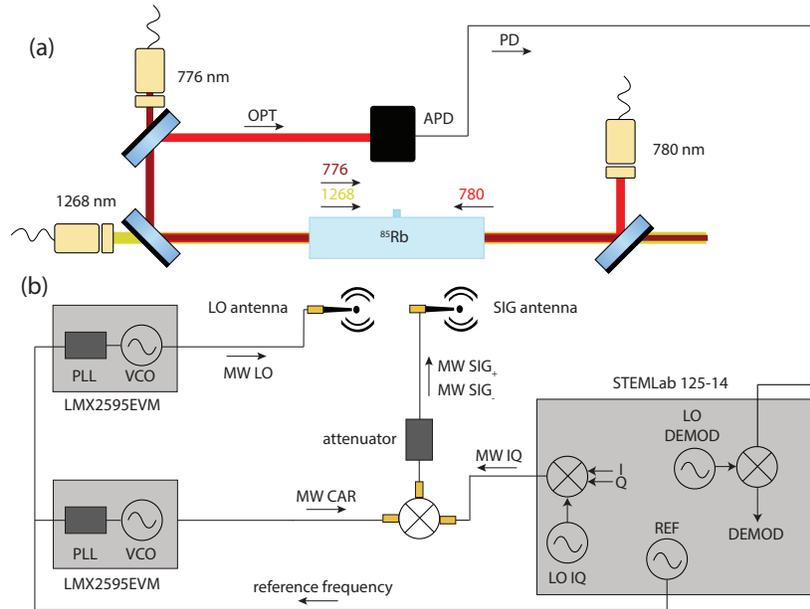
Fig. 2. (a) Optical part of the experimental setup. APD - avalanche photodiode, OPT - optical signal, PD - photodiode signal (b) The electronic part of the experimental setup. PLL - phase-locked loop, VCO – voltage-controlled oscillator, LO - local oscillator, MW - microwave, CAR - carrier signal, DEMOD - demodulation signal.
