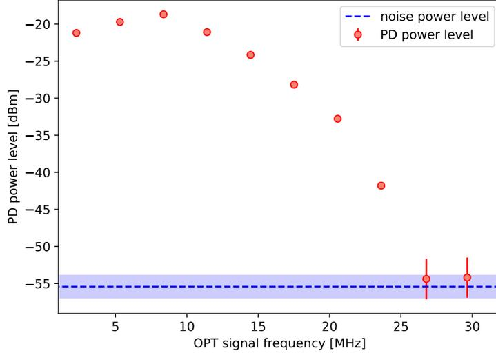
Fig. 6. Atomic response to the MW field in the case of heterodyne detection as a function of frequency of the OPT signal. The blue area around the line representing the shot noise power level corresponds to the error of the value of the noise power level.
