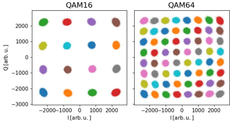
Fig. 7. The received points for the symbol frequency 122 kHz for the QAM16 and QAM64 schemes.
