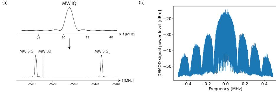
Fig. 3. (a) Spectra of the exemplary IQ signal used in the data transmission (upper spectrum), and signals sent from both antennas (lower spectrum). (b) Exemplary spectrum of the DEMOD signal in case of receiving quadrature amplitude modulated signal.
