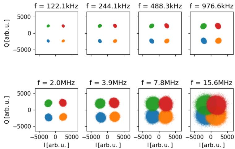
Fig. 8. The received points for QAM4 scheme for different symbol frequencies.
