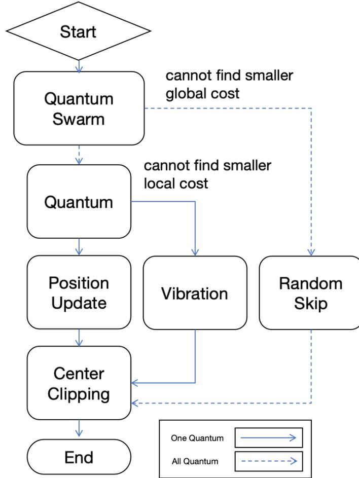
Fig. 1. Flowchart of One Iteration in HEO
