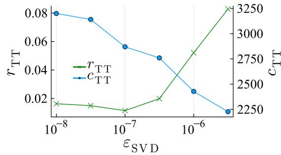
Figure 4: The maximum relative error  $r_{\text{TT}}$  and computational complexity  $c_{\text{TT}}$  when applying SVD with various  $\epsilon_{\text{SVD}}$  values to the TTs under the parameter settings of  $d = 10, \bar{\sigma}, \eta = \text{auto}$ . The left vertical axis represents  $r_{\text{TT}}$ , while the right vertical axis shows  $c_{\text{TT}}$ .
