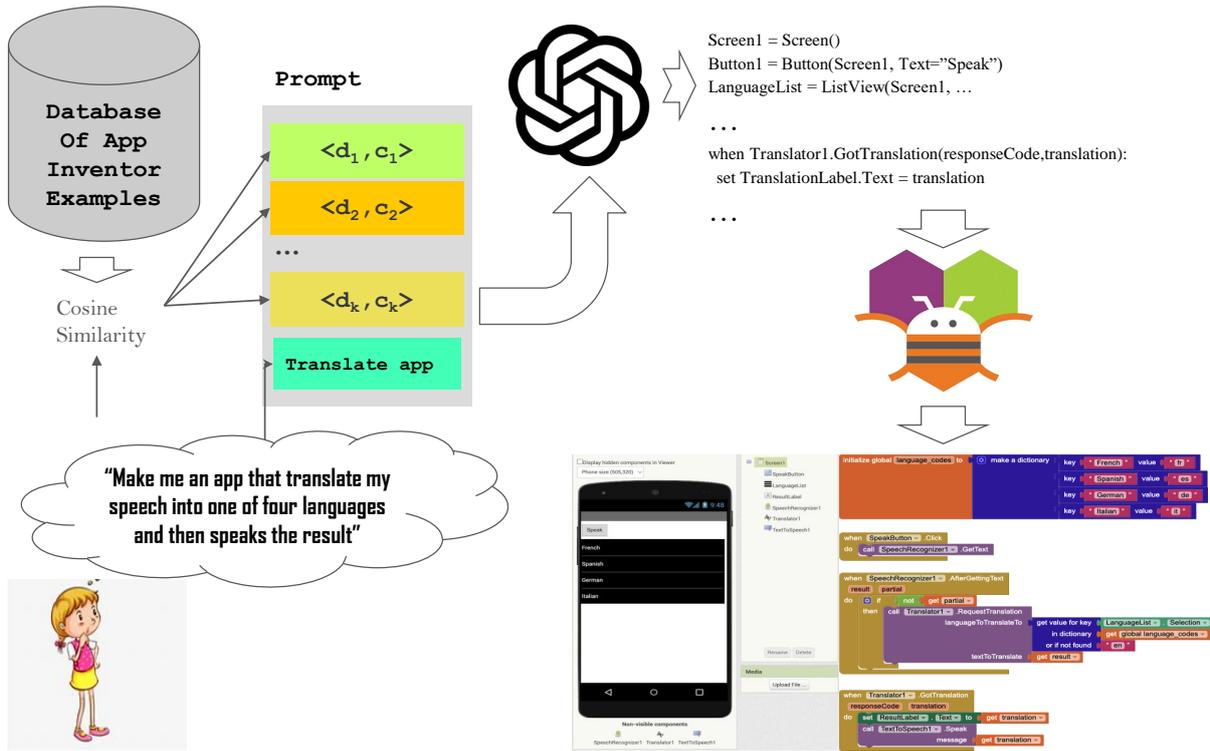
Fig. 3. When the user requests an application with its textual description, we automatically synthesize the prompt by adding several example pairs along with the desired application’s textual description. This constructed prompt is fed into one of OpenAI’s GPT-X models as an input, which outputs code that can be converted into a fully functional mobile application
