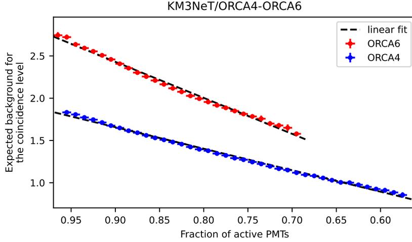
**Figure 2.** expected background of the coincidence level as a function of the fraction of active PMTs for ORCA4 (blue) and ORCA6 (red). The crosses indicate averaged values over the full periods, and the dashed lines are linear fits to these points.
