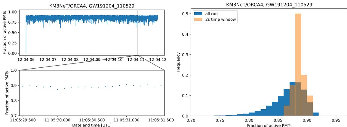
**Figure 4.** Time series (left) and distribution (right) of the fraction of active PMTs for the run covering GW191204.110529. On the left, the top plot shows the variability of the fraction of active PMTs during the run while the bottom plot is a zoom on the 2s time window starting from the GW event time. On the right, the distribution of the fraction of active PMTs is shown in blue for every timeslice of the run and in orange for the 20 timeslices inside the 2s time window.
