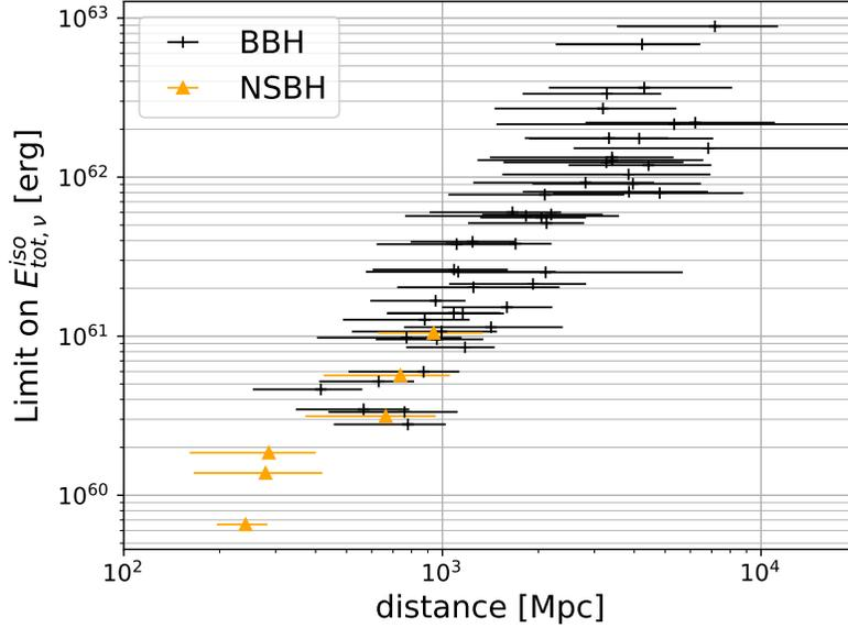
**Figure 8.** 90% upper limits on the total energy  $E_{\text{tot},\nu}^{\text{iso}}$  emitted in neutrinos assuming a quasi-thermal distribution centered at 13 MeV, as a function of the source luminosity distance, assuming an  $E^{-2}$  spectrum and isotropic emission.
